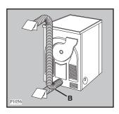
Once connected to the dryer, run the vent hose to the desired outlet point, ensuring that the run's overall length is less than 2 m, and that it contains no more than two bends. As to the outlet itself, if you have decided on a fixed wall/window grille, a good local builder's merchant should be able to supply you with the necessary fittings and installation advice.
